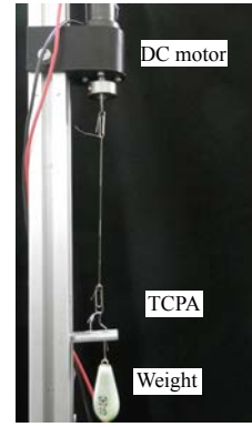
Fig.2 Fabrication machine of TCPA.
