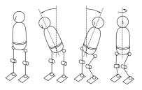
Figure 2: Bending motion of upper body with hip, knee and ankle joints
