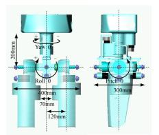
Figure 5: Demensions of the designed double spherical hip joint
