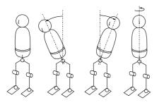
Figure 4: Bending motion of upper body with double spherical hip joints
