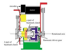
Figure 10: Design of the knee joint
