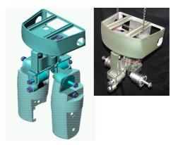
Figure 6: Photo of the double spherical hip joint
