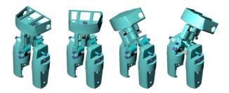
Figure 7: Trunk motion with the double spherical hip joint
