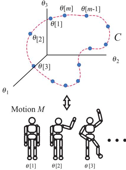
**Figure 1:** Robot posture, motion in the joint space
