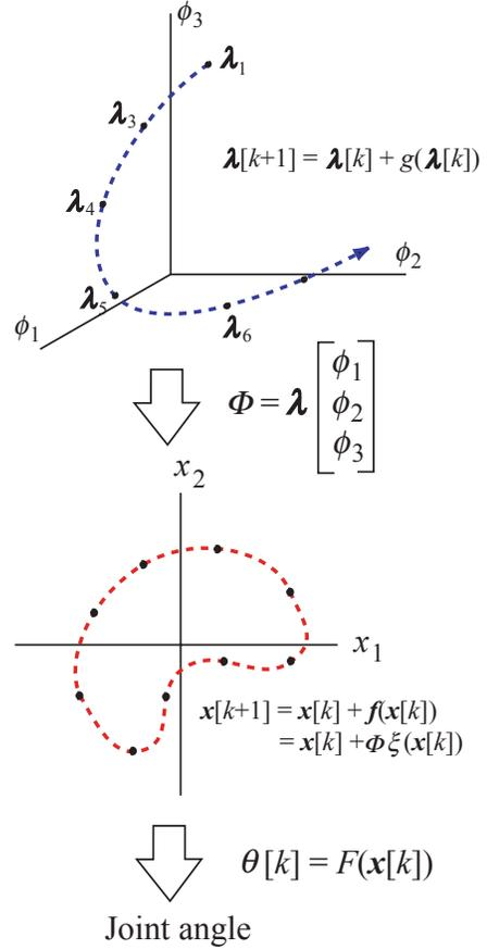
**Figure 4:** Connection of the symbol space and the motion space
