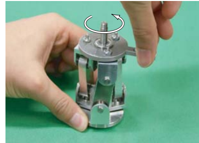
Fig. 4. Twist motion of the designed mechanism
