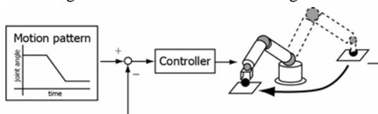
**Figure 1:** Motion control system for industrial robots
