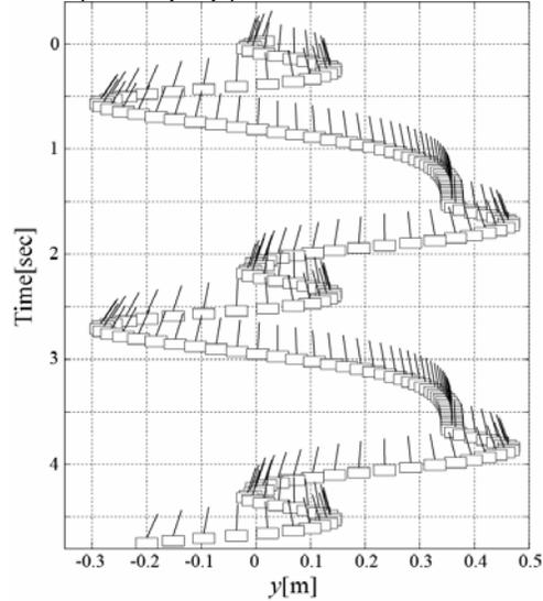
**Figure 6:** Reference motion pattern of the inverted pendulum system in the real world
