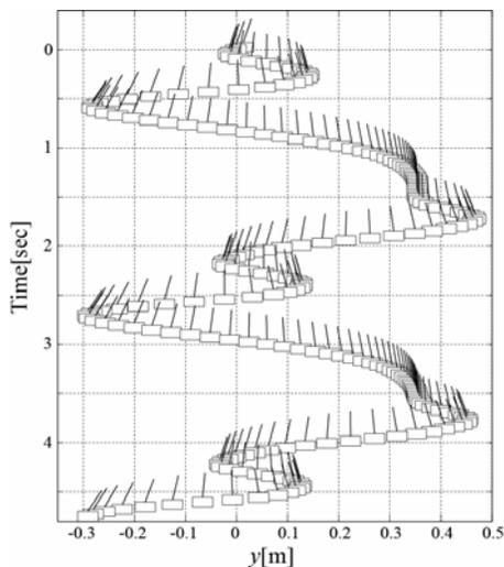
**Figure 19:** Motion of the inverted pendulum system via energy distance method
