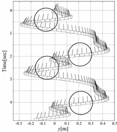
**Figure 10:** Motion of the inverted pendulum system in the real world with conventional method
