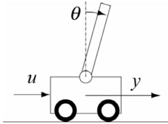
**Figure 4:** Inverted pendulum system
