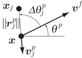
Fig. 4. Parameter definition for collision avoidance
