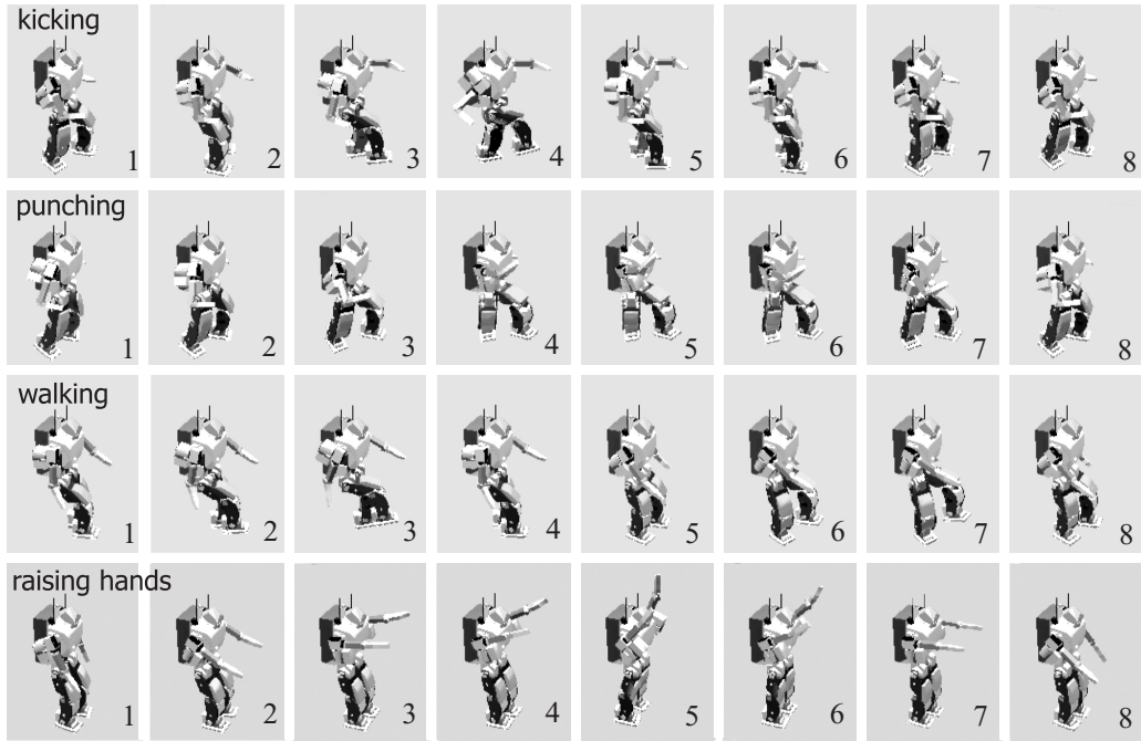
図 9 Generated motion of the humanoid robot
