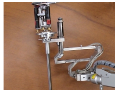
Fig. 2: Active Trocar with Closed Kinematic Chain
