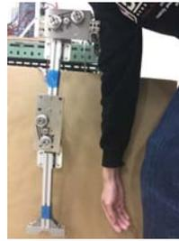
Fig.6 Two-degree-of-freedom robot
