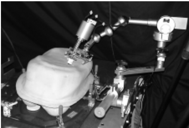
Fig.4 Slave Robot Positioning with Point-Setter
